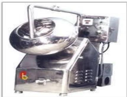
Fig. 4: Standard coating pan
