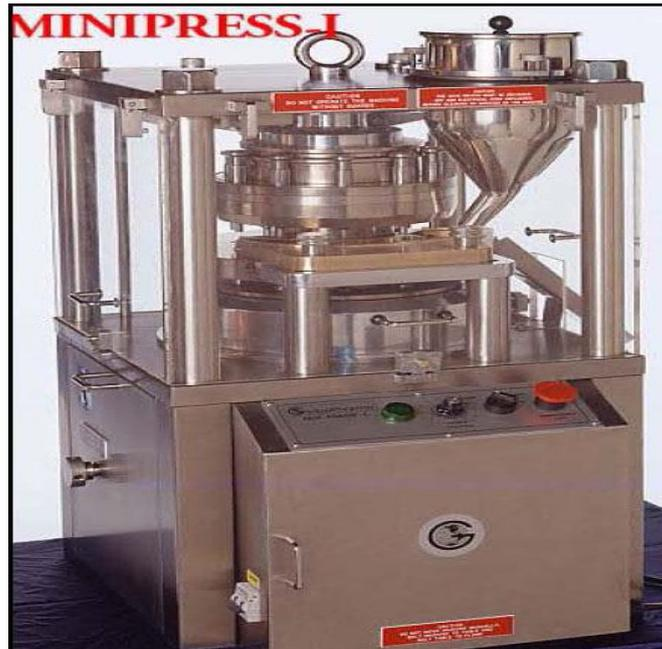
Fig. 3: Rotary Punching Machine
