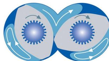
**Working principle of co-rotating twin screw extruder**
